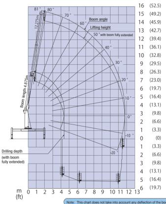
This chart assumes that the machine is set on firm level ground. The working range is 190 degrees to the rear of the vehicle.
